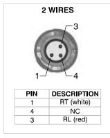
Socket for Power Supply STRAIGHT CONNECTOR M12A 4P FEMALE
