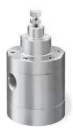
TESCOM 26-2900 Series is a dome loaded, negative bias, backpressure tracking regulator with a balanced main valve. This regulator controls upstream pressures up to 1000 psig / 69.0 bar with spring bias setting.
