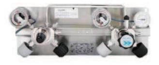
TESCOM Ultra High Purity Compact Panel is a VCR® compatible central gas supply unit for pressure control of high grade analytical gases in laboratory facilities. Depending on the requirements, these units switch over to a spare cylinder in order to enable an uninterrupted gas supply. The use of contact gauges allows the monitoring of empty gas cylinders, in combination with an annunciator.
