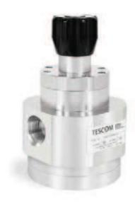
TESCOM DG Series single-stage regulator provides a compact size with high flow capability greater than 1000 SCFM / 28,300 SLPM. The large diaphragm and balanced main valve design provide lower droop (larger usable flow range) than competitive designs. Available in spring or dome loaded configurations.
