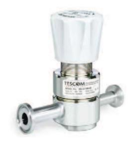
TESCOM PH-2200 Series is part of our Pharmpure™ product line. This high purity single-stage regulator offers a compact, USP Class VI and BPE compliant design suitable for specialty, corrosive, and pyrophoric gases of < 5 SCFM / 142 SLPM. Diffusion-resistant metal diaphragm seal ensures gas purity and integrity.
