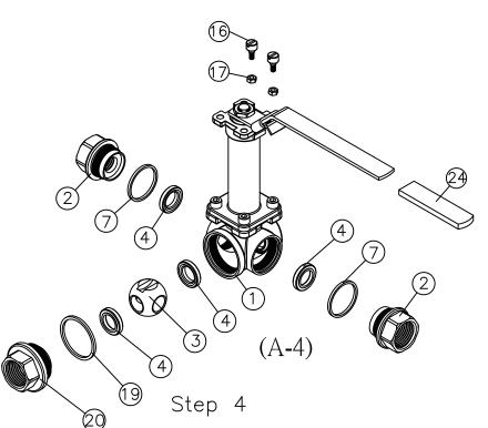
Fig (A-4) Put parts (4)(3) into (1) valve body.
