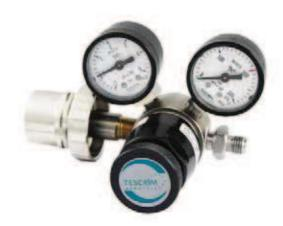
TESCOM WEGA Mini is a cylinder pressure reducer for gas purities up to 6.0 (99.9999 Vol %) used for lecture bottle and mobile applications. Lightweight and compact design due to the relief valve integrated into the body.
