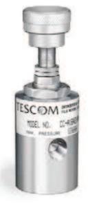
TESCOM CC Series metering valve is rated to 10,000 psig / 690 bar and contains a non-rotating stem to reduce seat and stem wear. The valve features over 20 turns from shutoff to full open, providing excellent flow control.
