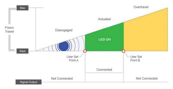
Figure 15. Dual Point Calibration Graph
