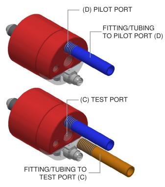
Figure 5. Attachment of Lines
