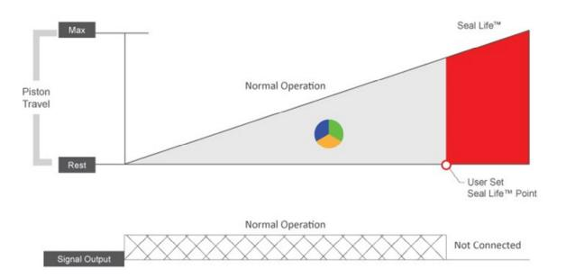
Figure 16. Seal Life™ Calibration Graph
