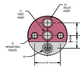
Figure 3. Connector Dimensional Features
