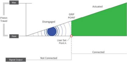
Figure 14. Single Point Calibration Graph
