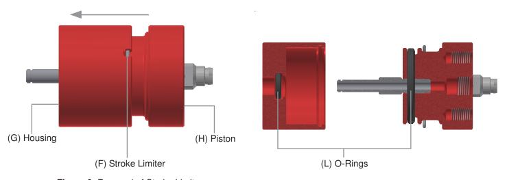
Figure 9. Removal of Stroke Limiter
