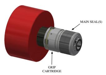
**FIG** Connectors provide a reliable leak-tight connection that grips and seals female ports. Simply insert male end of connector into female port, apply pilot pressure and then apply termination pressure.
