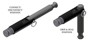
The Jaws JNL Connectors provide a reliable leak-tight connection that grips and seals in holes and ports. Simply place the JNL connector into a port, activate the mechanical gripping and sealing action, then introduce the test media. For vacuum to 1000 psi applications with air, gas, or liquid, Fastest JNL Connectors provide secure, leak tight sealing for manual connections.
