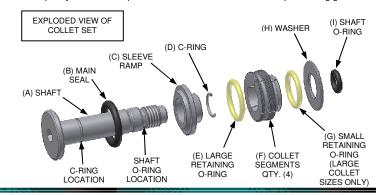
4. Assemble the collet segments (F) and retaining o-ring(s) (E) & (G). Arrange the four pieces of collet (F) into a circle with the raised area facing upward. Place the retaining o-ring(s) into the groove(s) on the raised area.
