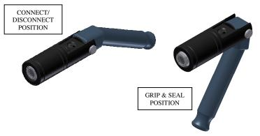
**Nuclaws** JXL Connectors provide a reliable leak-tight connection that grips and seals straight tubing. Simply place the JXL connector onto a tube, activate the mechanical gripping and sealing action, then introduce the test media. For vacuum to 1000 psi applications with air, gas or liquid, **Fastest Nuclaws** JXL Connectors provide secure, leak tight sealing.
