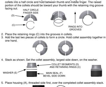
1. First step, assemble collet segments (D) and retaining rings (C), form two pieces of
