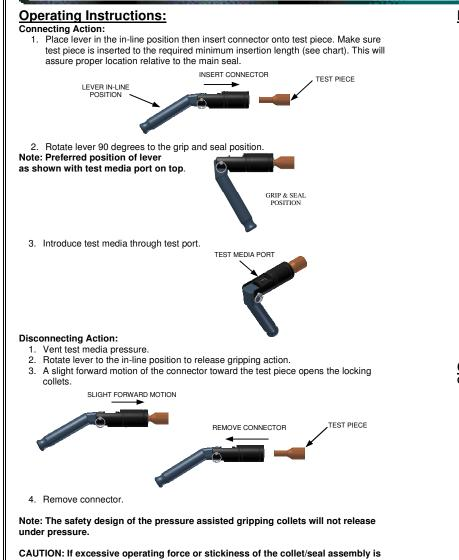
CAUTION: If excessive operating force or stickiness of the collet/seal assembly is noted, remove collet/seal assembly (See Collet Set Removal and Installation:) and check for alignment and lightly lube the bore of the housing with a petroleum jelly or other compatible lubricant.
