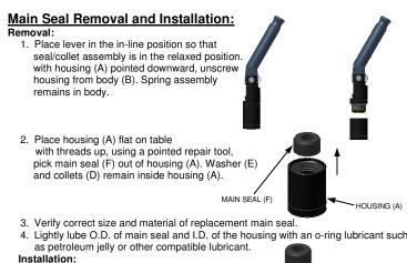
Place replacement main seal (F) bevel side up into housing and slide it down against washer (E).
