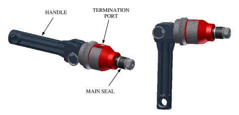
**ZN** Connectors provide a reliable leak-tight connection that seal on smooth bores. Simply insert male end of connector into bore and rotate handle to engage seals to bore.
