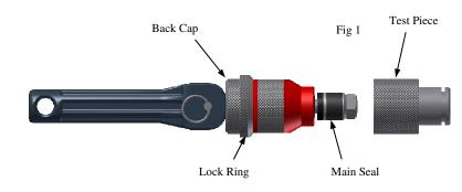
4. Insert connector into port and rotate handle 90° degrees in either direction. Main seal is compressed as handle is rotated.
