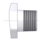
NPT Female Threads acc. to ASME B 1.20.1
