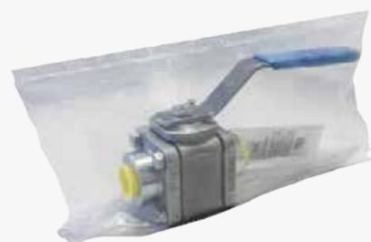
The valves can be degreased to achieve high levels of cleanliness and prevent hydrogen autoignition in service. Afterwards this the valves are packed and sealed in individual protective plastic bags with silica to prevent contamination and humidity problems.
