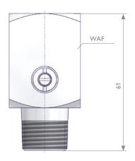
Gauge Snubber Type made from 32 mm square barstock material.
