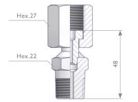
Max. allowable (Working) Pessure (PS): Type 1 10,000 psi / 689 bar Type 2, 3, 4 6,092 psi / 420 bar
