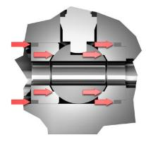
The forces required to maintain the tightness are stressing all components - even the ball and ball seats. The operating torque is thus very high.
