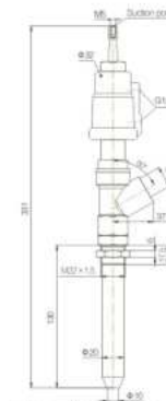
1AP Filling Valve with Internal Sealing and Suction
