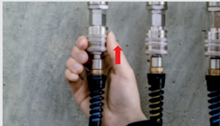
Disconnection - first step: Automatic venting
