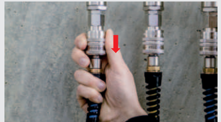
Disconnection - second step: Safe decoupling
